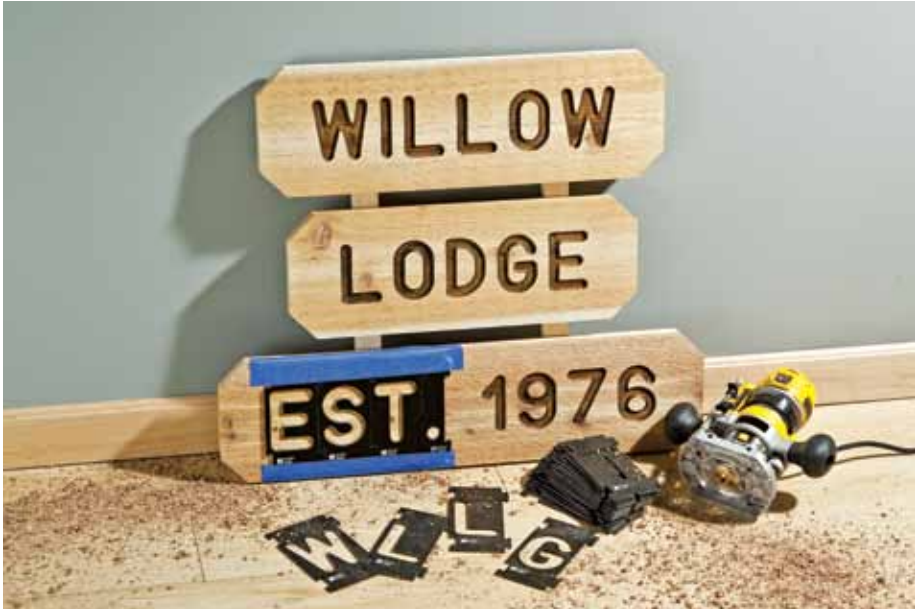
Unique two template system eliminates center islands leaving perfectly routed letters.
